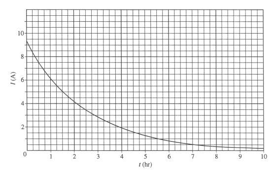
The equation for this curve is  $I = I_0 e^{-kt}$ , where t is the time elapsed from the instant the switch is closed and  $I_0$  and k are constants.
