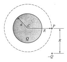
A point particle of charge -Q is now placed a distance R below point P, as shown above.
